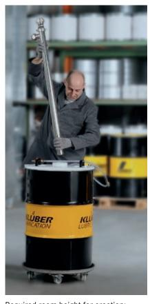
Required room height for erection: Approx. 86.6" (2200 mm), without motor
